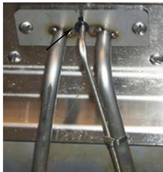
Pull old probe wire through grommet to remove probe.
